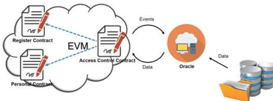
Figure 2. The sketch map of the proposed access control system (ACS) for protecting sensitive databases. [1]
