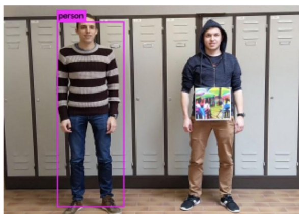
Figure 3: An illustration of the adversarial patch based attack
