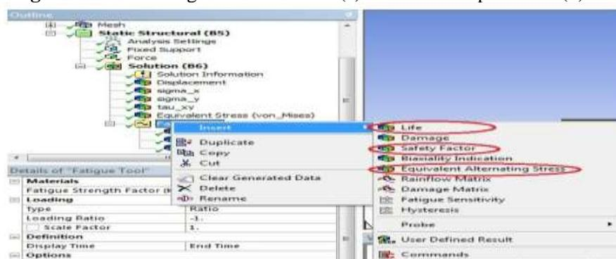
Figure 2 Different options in the Fatigue Tool
